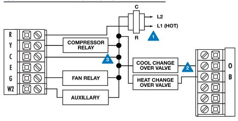
**NOTE:** In many systems with no emergency heat relay a jumper can be installed between E and W2.
